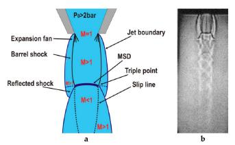
**Figure 1.** Scheme (a) and shadowgraph image (b) of the free jet emerging from a conical nozzle commonly used in laser fusion cutting for an operating parameter range  $P_0/P_a > 1.89$  (Riveiro *et al.*, 2019)
