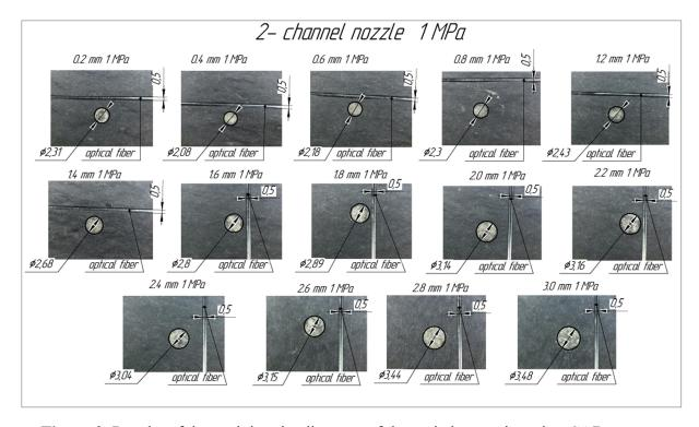
Figure 3. Results of determining the diameter of the assisting gas jet using CAD system
