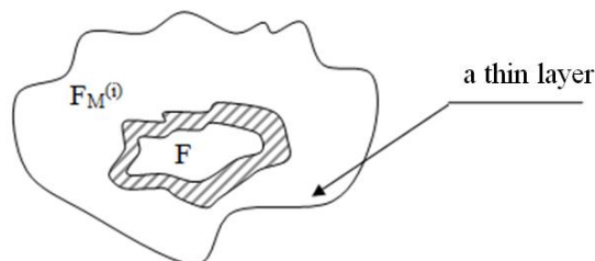
Figure 1 – Model of contact of two bodies in view of the interface
