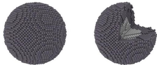
Fig. 1. Initial atomistic configuration of Ag@Pd core-shell nanoparticle: overall view (left panel) and cross-section (left panel). Pd atoms (shell) are shown in dark gray color; Ag atoms (core) are shown in light gray color.
