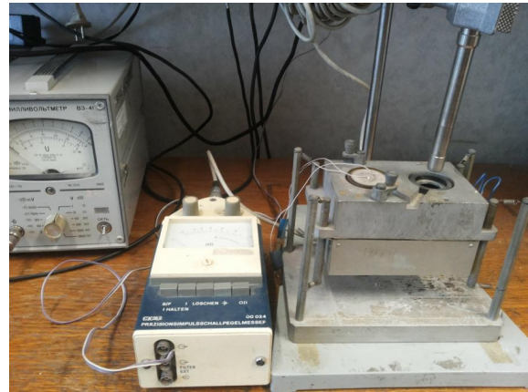
Figure 8 – Experimental stand with vibroacoustic chamber
