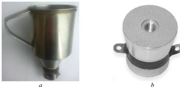
Fig. 1. Laboratory stand (*a*) for intensification of chemical processes based on Langevin's radiator (*b*)
