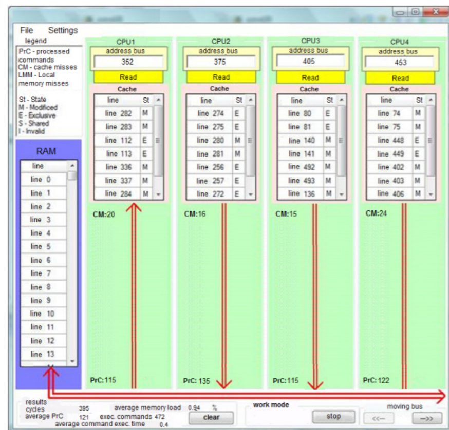
Fig. 7 System without local memory structure
