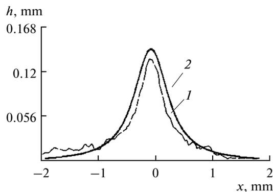
Fig. 7. (1) Experimental and (2) calculated profile of a groove (the wire's diameter is 0.15 mm, the IEG is 0.3 mm, and  $\Delta\phi = 4$  V).
