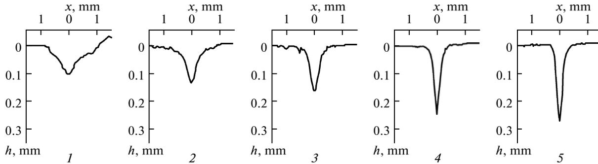
Fig. 6. Profilograms of the processed plate obtained when using a wire diameter of 0.15 mm. Δ: (1) 0.5, (2) 0.3, (3) 0.2, (4) 0.1, and (5) 0.05 mm.
