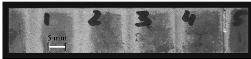
Fig. 5. Image of the processed plate obtained when using a wire with a diameter of 0.15 mm. Δ: (1) 0.5, (2) 0.3, (3) 0.2, (4) 0.1, and (5) 0.05 mm.
