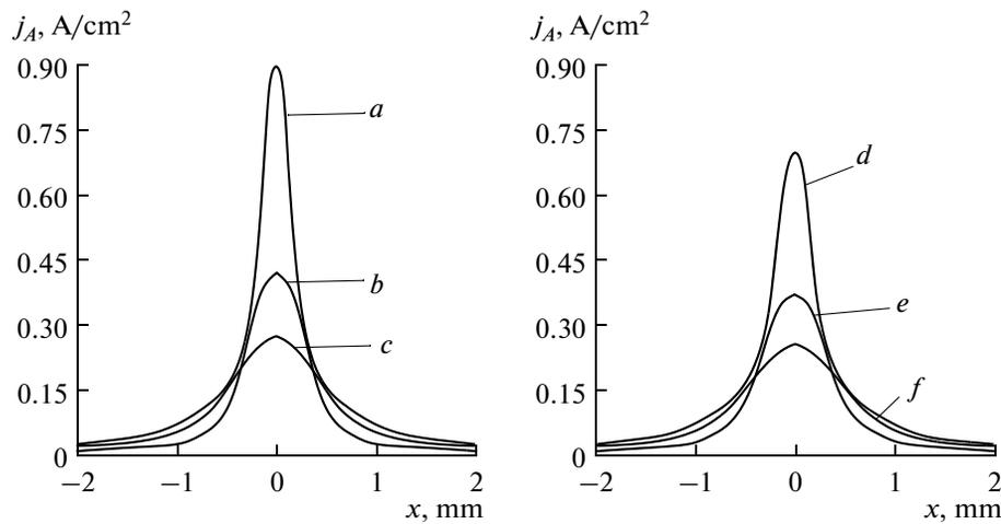
**Fig. 3.** Distribution of the anode current density over the anode surface in processing by electrodes with diameters of (a)–(c) 0.15 and (d)–(f) 0.25 mm for  $\Delta =$  (a), (d) 0.1; (b); (e) 0.3; and (c), (f) 0.5 mm (6% aqueous NaCl solution with the specific conductivity  $\kappa = 0.0871/(\Omega \text{ cm})$ ).
