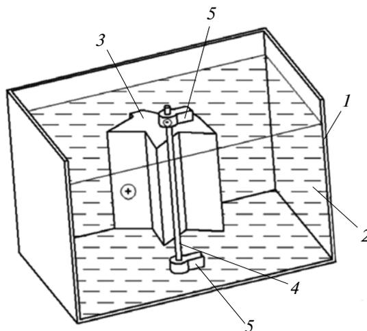
**Fig. 1.** WEECP scheme: (1) working electrolyte bath, (2) electrolyte, (3) workpiece under treatment, (4) wire electrode, and (5) wire electrode holders.
