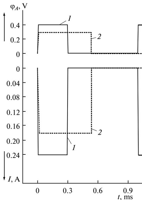
**Fig. 4.** Rectangular-shaped oscillograms of the anode polarization by the currents (the cathode is the wire DKRPM FKTL-63 electrode,  $\varnothing 0.15$  mm). The value of the interelectrode gap is as follows: (1) 0.3 and (2) 0.5 mm. The duration of the current impulses is as follows: (1) 300 and (2) 500 ms.
