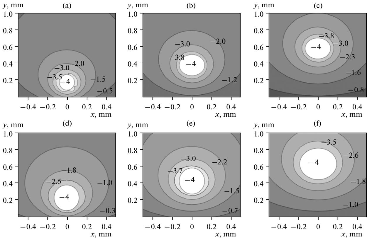
**Fig. 2.** Isopotential lines in the interelectrode gap between the cylindrical wire electrodes with diameters of (a)–(c) 0.15 mm and (d)–(f) 0.25 mm and the flat workpiece’s surface for the following magnitudes of IEG: (a), (d) 0.1; (b), (e) 0.3; and (c), (f) 0.5 mm (at a potential difference between the electrodes of 4 V with considering the anodic and cathodic polarization).
