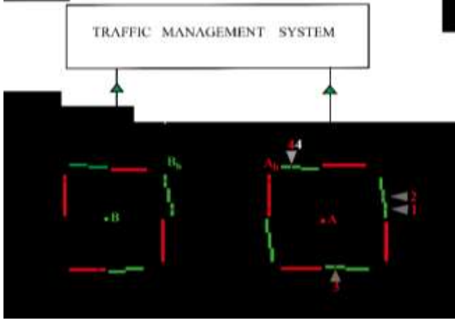
Fig.1. – Two adjacent cross-shaped intersections – A and B –and vehicles that enter the lane between these intersections are shown. The red stripes are input sensors. Output sensors are represented as three adjacent green stripes. The vehicle route of a number 4 is shown.
