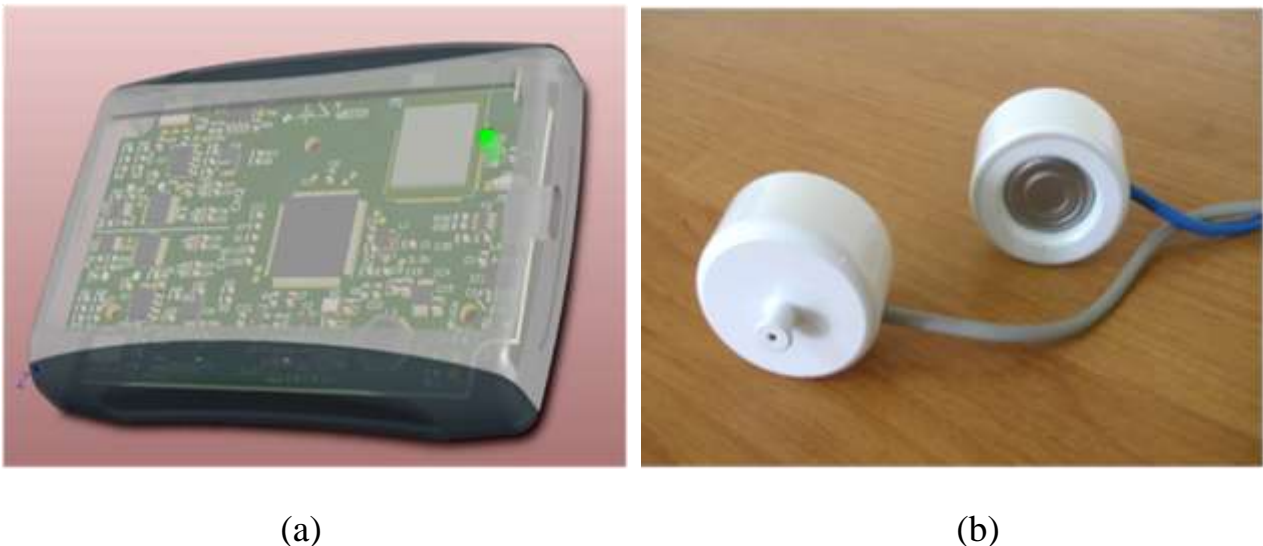
Figure 12. Constructive realization of the microcontroller block (a) and PRMT of surplus pressure (b)
