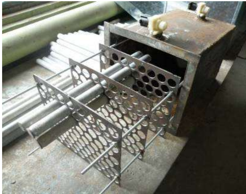
Figure 4. The first design option of the experimental sample – with capsules of heat-accumulating substance.
