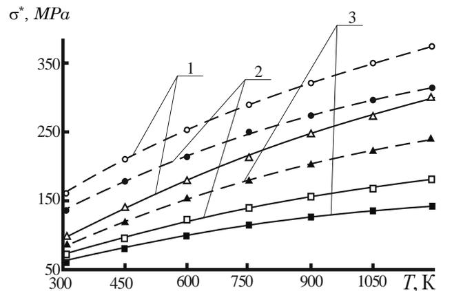
**Fig. 6** – Dependencies of values of maximum thermoelastic stresses in the elements of optical ceramics KO1 (1), KO2 (2), KO3 (3) from the heating temperature ( $P = 10^5 \text{ Pa}$ , thickness of the element  $H = 4 \cdot 10^{-3} \text{ m}$ ,  $F_n = 1.6 \cdot 10^7 \text{ W/m}^2$ ,  $V = 10^{-3} \text{ m/s}$ ): — — — elements unprocessed by electron beam; - - - - processed elements;  $\Delta, \circ, \square, \blacktriangle, \blacksquare, \bullet$  – experimental data.
