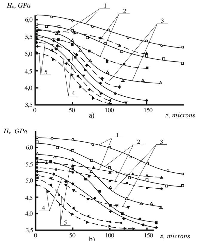
**Fig. 2** - Dependencies of microhardness at the depth of elements of optical ceramics KO12 (1), KO2 (2), KO1 (3), KO3 (4) and KO5 (5), processed by electron beam: a) - for different speeds of movement (— — —  $V = 7 \cdot 10^{-3} \text{ m/s}$ ; - - - -  $V = 1.5 \cdot 10^{-2} \text{ m/s}$ ) and  $F_n = 1.5 \cdot 10^7 \text{ W/m}^2$ ; b) - for different values of its thermal effect density (— — —  $F_n = 1.5 \cdot 10^7 \text{ W/m}^2$ ; - - - -  $F_n = 5 \cdot 10^6 \text{ W/m}^2$ )
