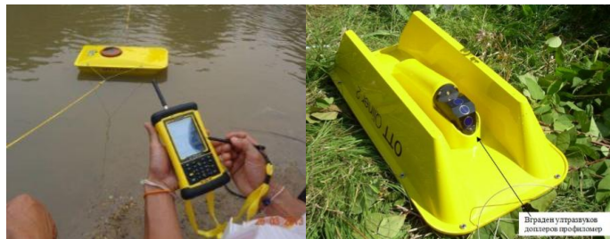
Fig.1 "Measurement of water quantity with hydrometric system –OTT Qliner 2
