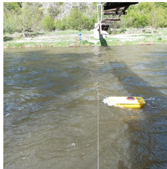
Fig.3 Measurement of water quantity with hydrometric system –OTT Qliner 2 the station №52800, place near to Gotse Delchev
