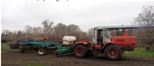
Fig. 2. - Experimental sample of the combined unit for cultivation and mulching of the soil with plant remains
