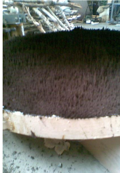
Fig. 4. Ferromagnetic powder after treatment with magnetic field
