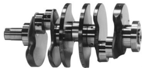
Fig. 4 Crankshaft of a four-stroke diesel engine [10]
