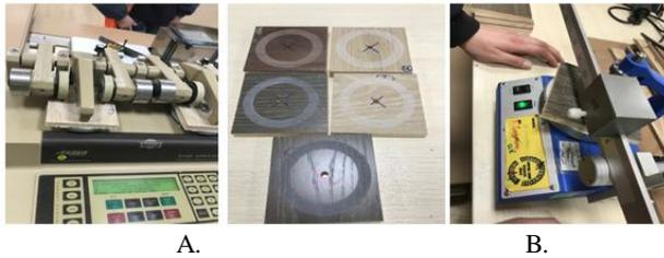
Figure 2. A. Surface abrasion test. B. Surface scratch test.
