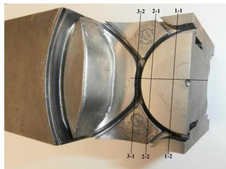
Fig.3 Sampling procedure from the mold part
