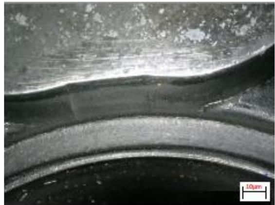
**Fig.1** Degradation of the mold part
