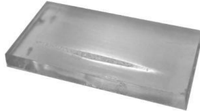
Fig. 2. Observed destructions of the elements from optical glass (K8, K108) and ceramics KO2 by exceeding the parameters of external actions of their critical values ( q_n^* , t^* ).
