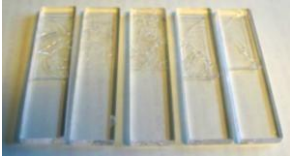
Fig. 2. Observed destructions of the elements from optical glass (K8, K108) and ceramics KO2 by exceeding the parameters of external actions of their critical values ( q_n^* , t^* ).
