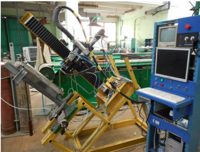
Fig. 4. Laboratory stand for laser welding of steels and alloys in different spatial positions.
