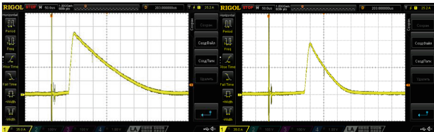
Fig. 5. Comparison of discharge currents obtained at spark gap lengths of 0.5 mm (left) and 13 mm (right). Division scales: current 35 A/div, time 50 \mu\text{s} /div.
