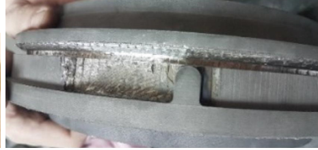
Fig. 2. Hard-to-remove massive part supports.
