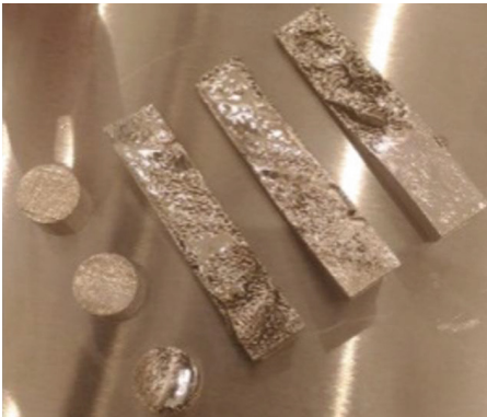
Fig. 5. The uneven penetration of the build area due to an uncalibrated laser.
