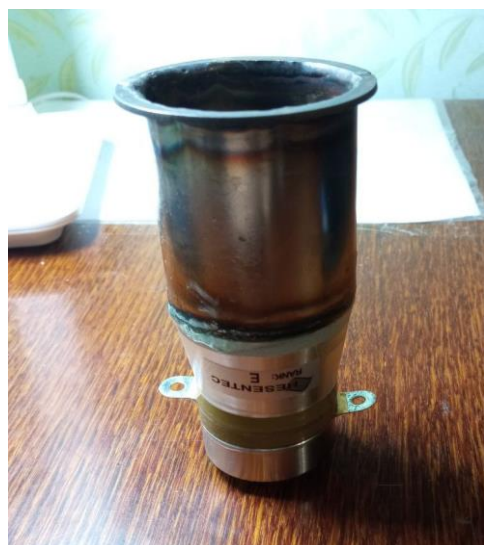
Figure 7. Experimental sample of ultrasonic system for extraction
