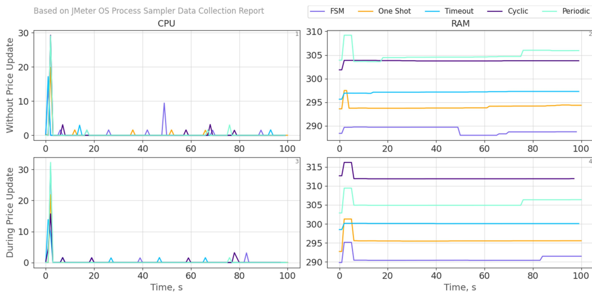
Figure 13. Line graphs for comparing the amount of consumption of hardware resources (CPU, RAM) for different SPADE agent behaviors (FSM, One Shot, Timeout, Cyclic, Periodic) during and outside the price update process
