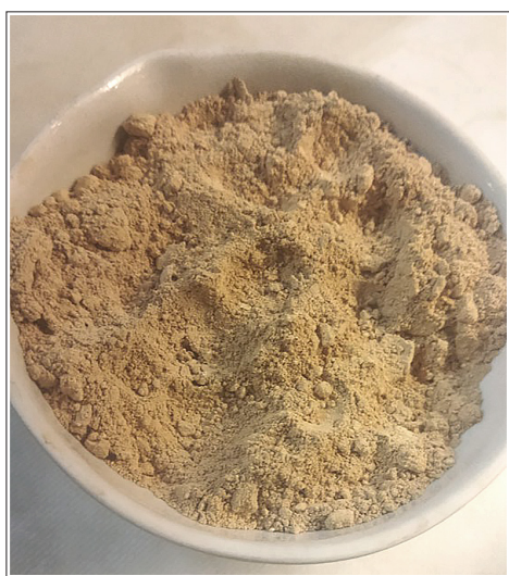
Figure 1. Cement additive obtained as a result of neutralisation of the mother solution from the contaminated filter
