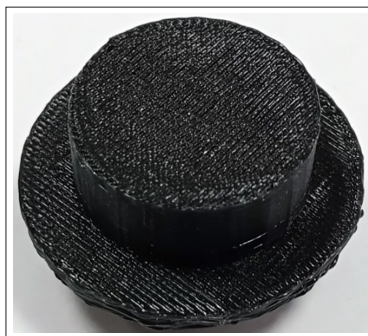
Figure 2. Exterior view of the product (Boeing Insitu ScanEagle (USA) UAV compressor bushing) printed by the curved layer method using solid layer 3D printing technology
