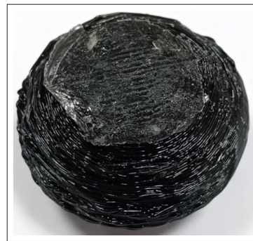
Figure 1. Exterior view of the product (Boeing Insitu ScanEagle (USA) UAV compressor bushing) printed by fused deposition using 3D printing technology with a distinct segmented texture effect
