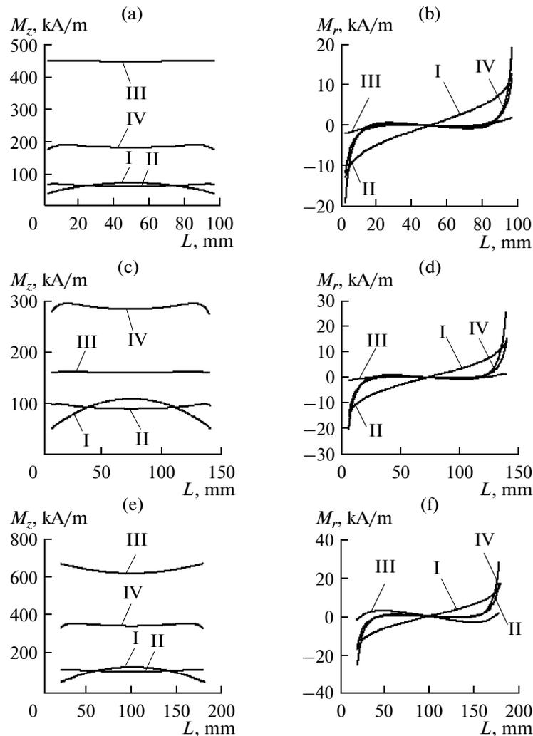
**Fig. 3.** Distribution of the axial and radial components of the sample magnetization along its length at the distance of 0.5 mm below its surface for the studied magnetization types and the following values of  $L$ : (a, b) 100; (c, d) 140; (e, f) 168 mm.
