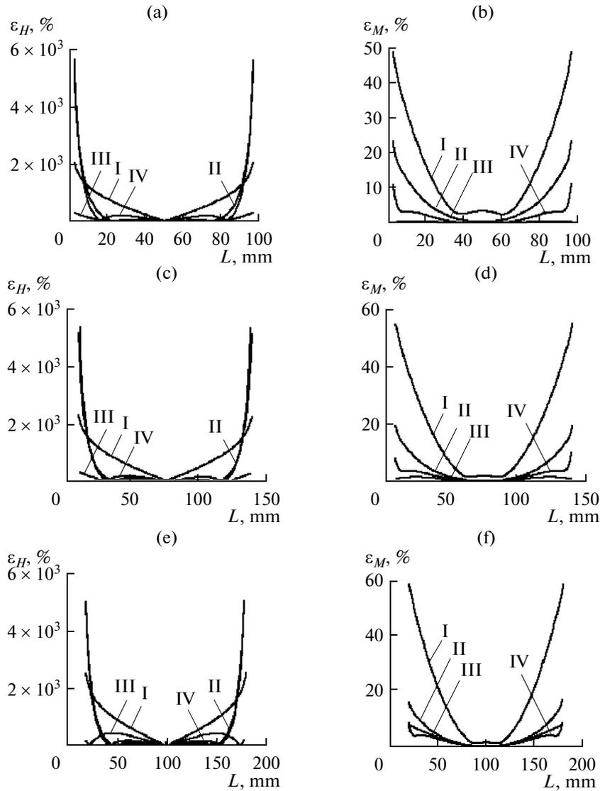
**Fig. 4.** The distributions of the errors in the homogeneity of the magnetic field intensity and magnetization vectors along the sample with respect to the centered value of  $H_c(M_c)$  and measured at a distance of 0.5 mm above and below its surface, respectively, for the  $L$  values of (a, b) 100, (c, d) 140, and (e, f) 168 mm.
