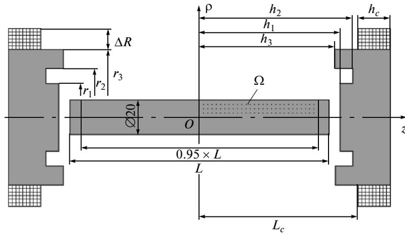
Fig. 1. The geometric model of the magnetization system with a sample.
