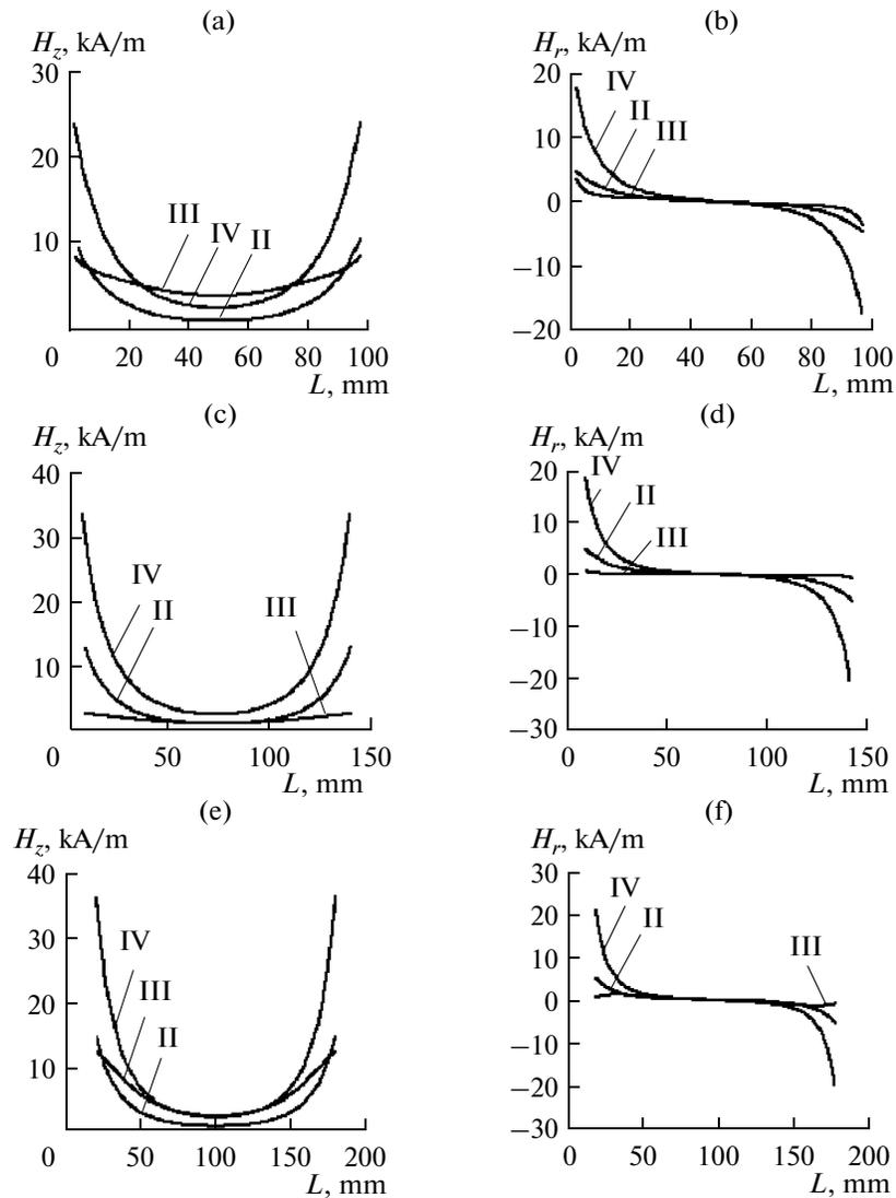
**Fig. 5.** The distribution of the axial and radial components of the magnetic field intensity of the synthesized source (magnetization types (II)–(IV)) in the control zone along the length of the imaginary sample at the distance of 0.5 mm above its surface and the  $L$  values of (a, b) 100, (c, d) 140, and (e, f) 168 mm.
