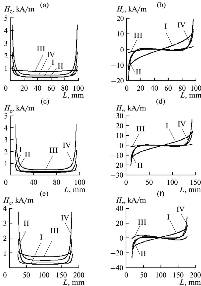
Fig. 2. Distribution of the axial and radial components of the magnetic-field intensity along the sample at a distance of 0.5 mm above its surface for the studied magnetization types and the following values of  $L$ : (a, b) 100; (c, d) 140; (e, f) 168 mm.
