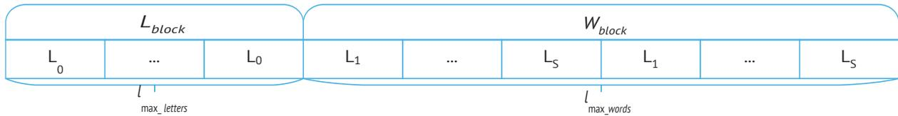
**Figure 3.** Structure of synchronisation block and data block
