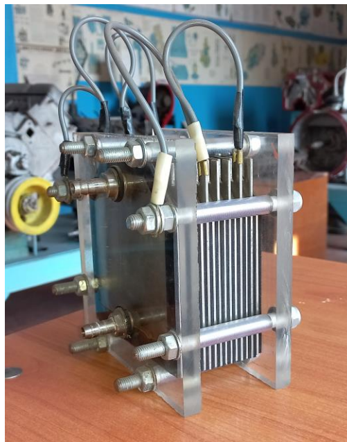
FIGURE 1. Device for production of hydrogen-containing gas (Electrolyzer)
