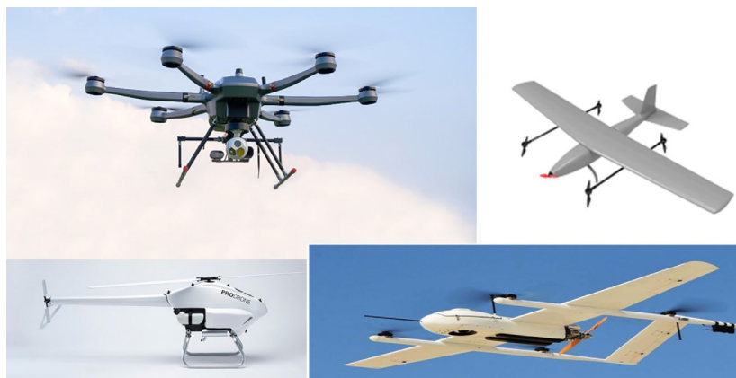
Figure 1. Main drone types: multi-rotor, fixed-wing, single-rotor and hybrid VTOL
