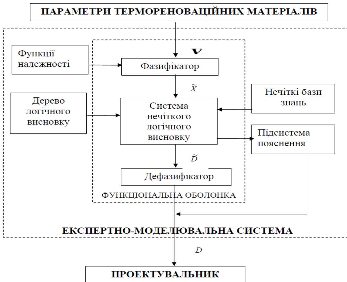
Fig. 1 – Structural model of management decision support for the choice of thermal renovation material
